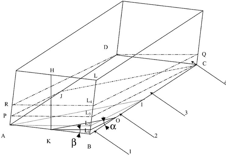
Fig. 2. The different zones (1, 2, 3, 4) of water filling (see text). Here,  $h$  is measured along  $KH$ ,  $h_0 = BL_1$ ,  $h^*$  is the water height along  $BL$ . The different zones correspond to the following volumes: (1)  $KBOL_1$ ; (2)  $ABIL_2$ ; (3)  $ABCJL_3$ ; (4)  $ABCDRL_4Q$ .
