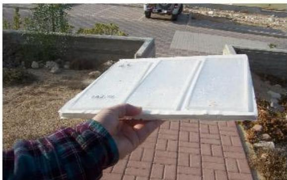
**Fig. 2** One of the prototypes of a "compact" condenser
